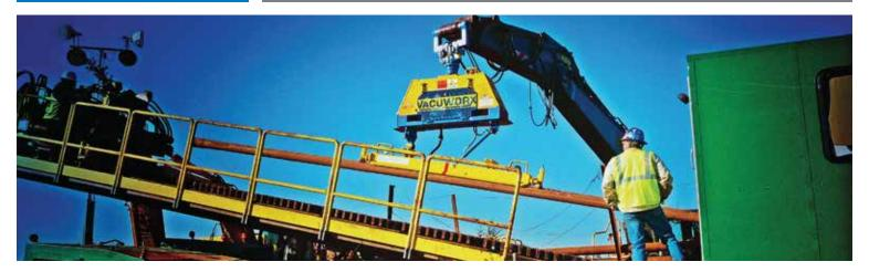
HDD PIPE LIFTING SYSTEM uses vacuum technology to lift drill stem and position it into the rig without the use of slings or personnel.
